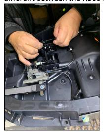
(5) Once installed, cut slits in the cover and reinsert factory clip which is still sewn to the carpeted board.
