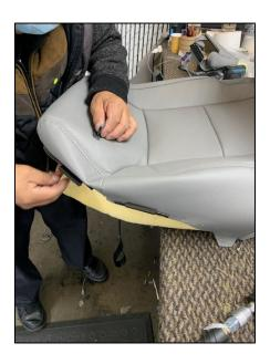
(3) Pull cover on and cut holes for headrest posts.
