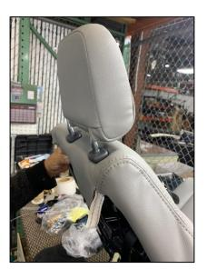
(4) Re-attach headrest cables and finish installing the covers. Make sure you install the correct rear headrest as the cables are different between the RB60 & RB40.
