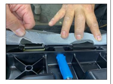
(7) Pull the release strap through the slot and attach original factory backboard to the frame.
